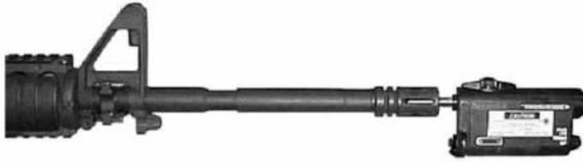
Figure 1. Borelight inserted properly (Battery Down).
