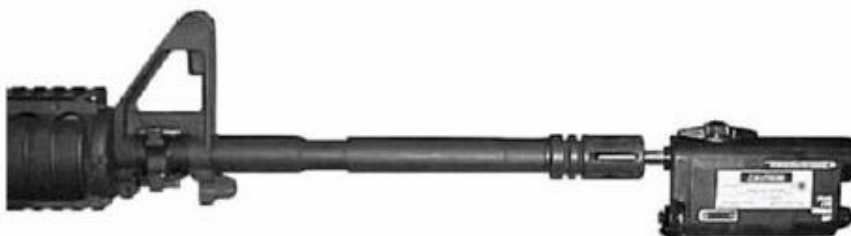
Figure 4. Rotating the Borelight (Half Turn/ Battery Down Position).
