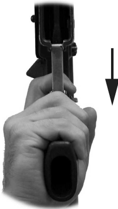
Figure 1 Proper Finger Placement
