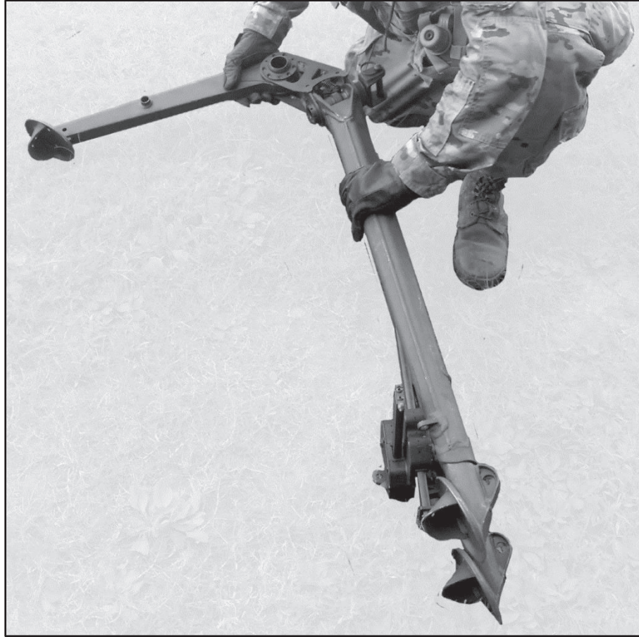
Figure C-2. Place front leg in the deployed position
