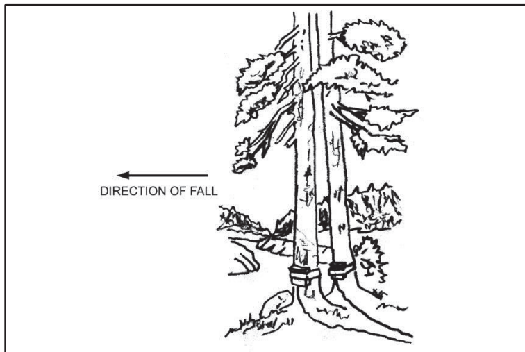
Figure 5-12. Timber-cutting charge (external)
