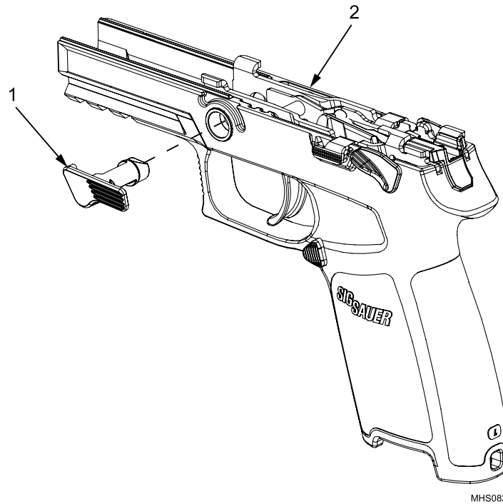
Figure 40. Takedown Lever Installation.
