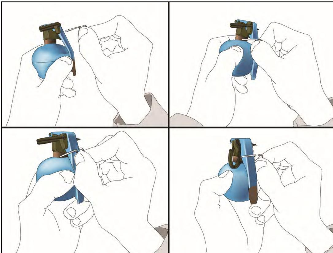
Figure B-4. Safety clip installation
