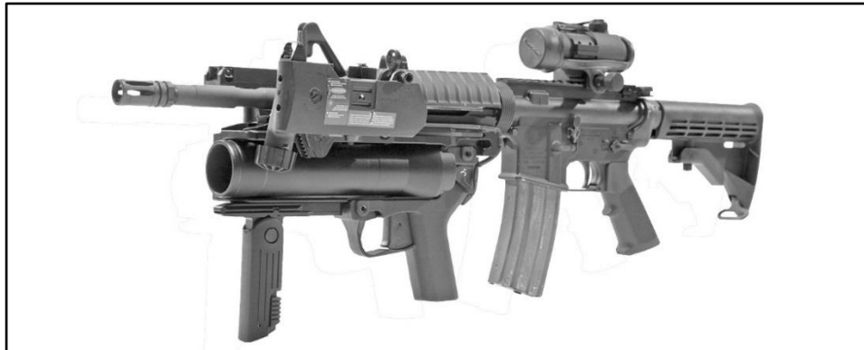
Figure 4-1. M320 attached to M4 series carbine example
