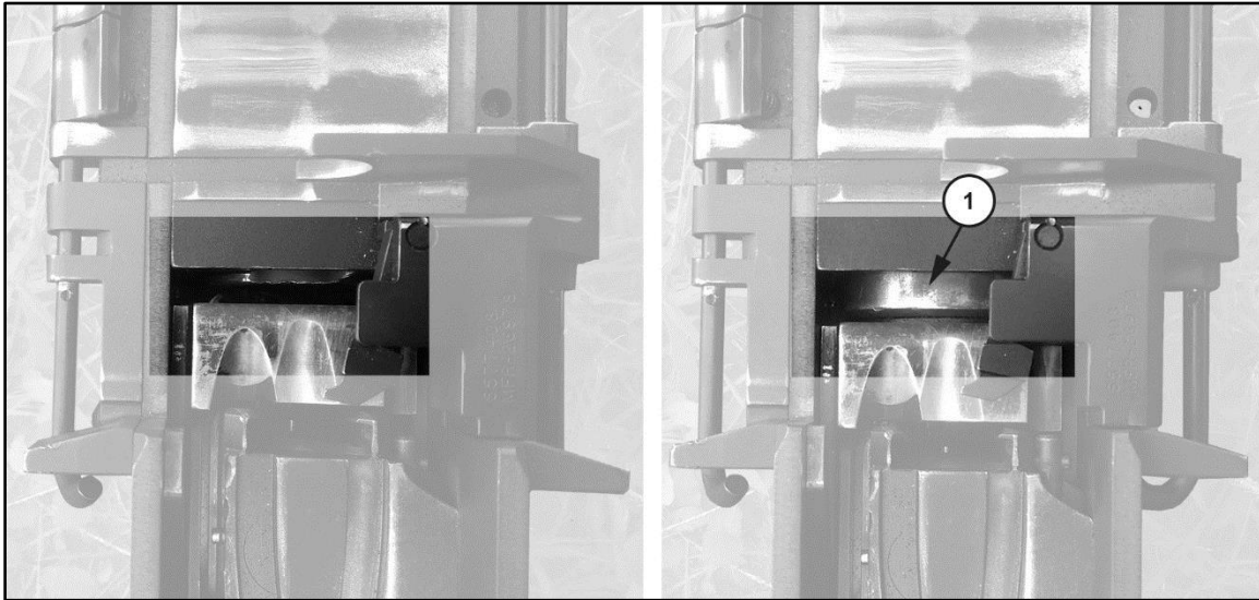
Figure D-14. Inspect barrel and barrel extension
