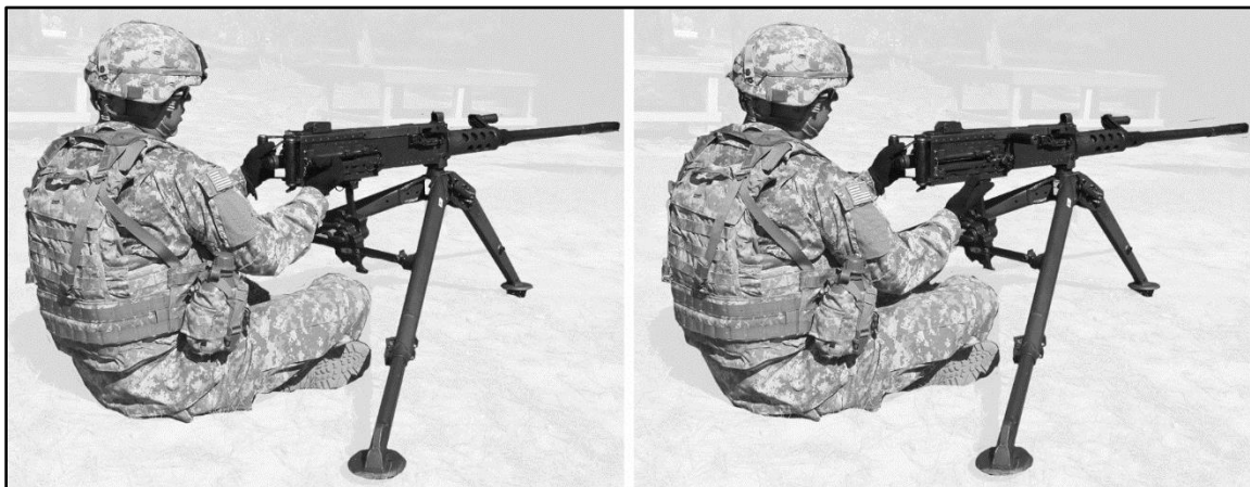
Figure D-16. Charge weapon to ensure barrel moves freely
