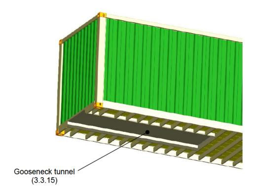
FIGURE 13. Container understructure
